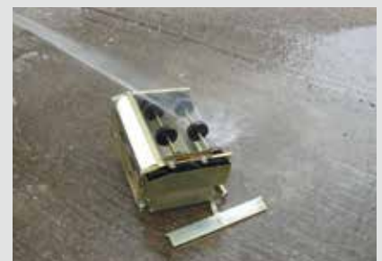
After work, the VD mortar roll is thoroughly cleaned with plenty of water.
