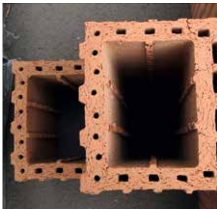
Layer by layer, projectile-high through-hole channels are created, which are then filled with concrete.
